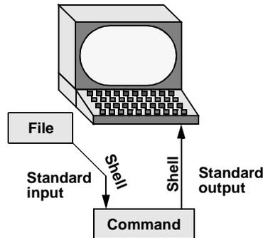
Figure 5-8 Redirecting standard input
