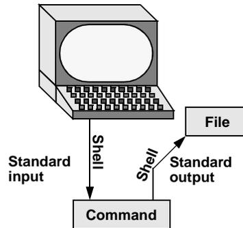
Figure 5-5 Redirecting standard output
